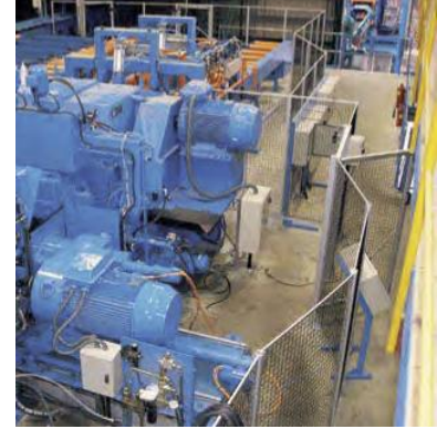
Quick-Guard E with few components and easy to angle at up to 45°.
