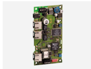
IP Converter add-in card with integrated switch for connecting digital Intercom Stations
