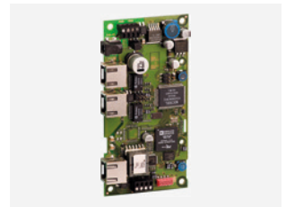
IP Converter add-in card with integrated switch for connecting analogue Intercom Stations
